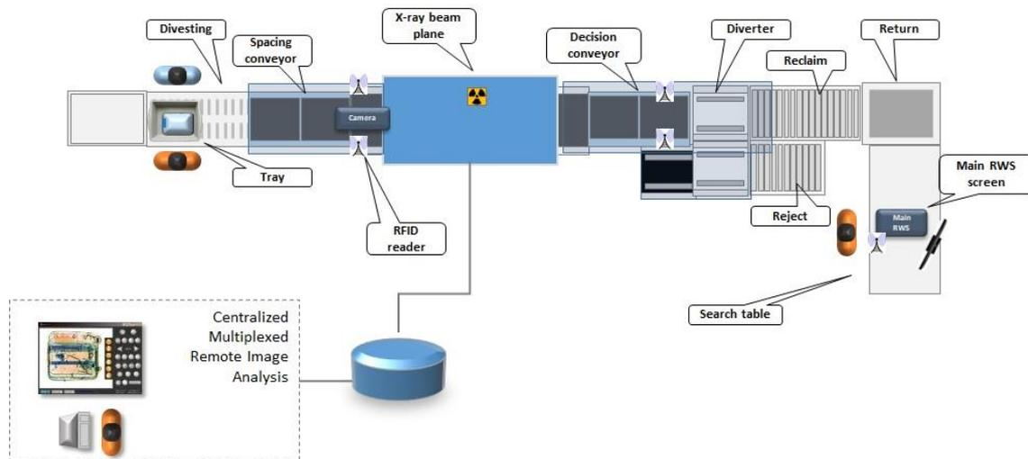
Figure 6. Remote screening checkpoint layout.
