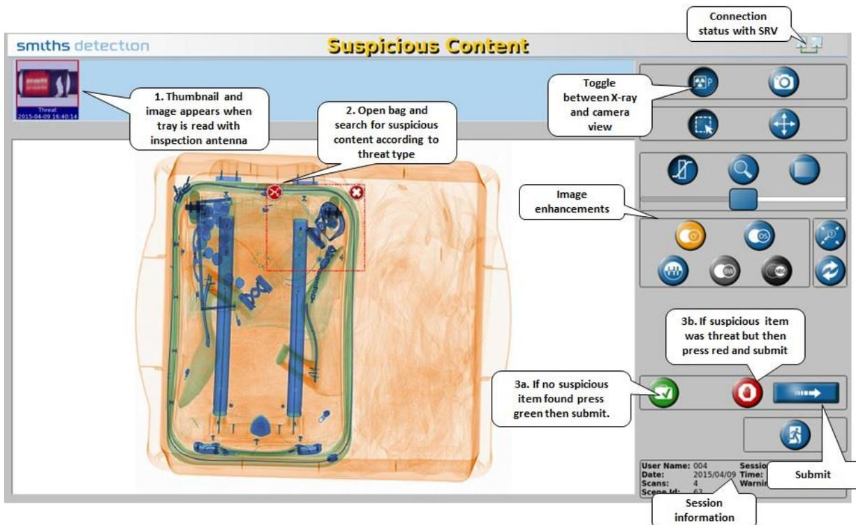
Figure 5. Recheck workstation – Graphical User Interface (GUI)
