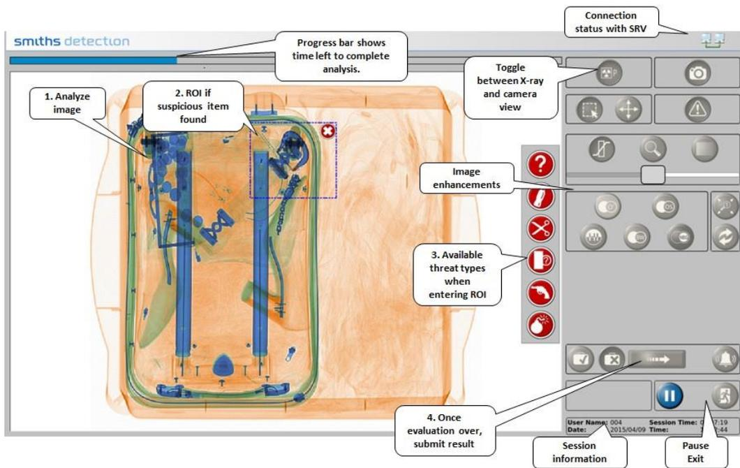
Figure 4. Analyst workstation – Graphical User Interface (GUI)
